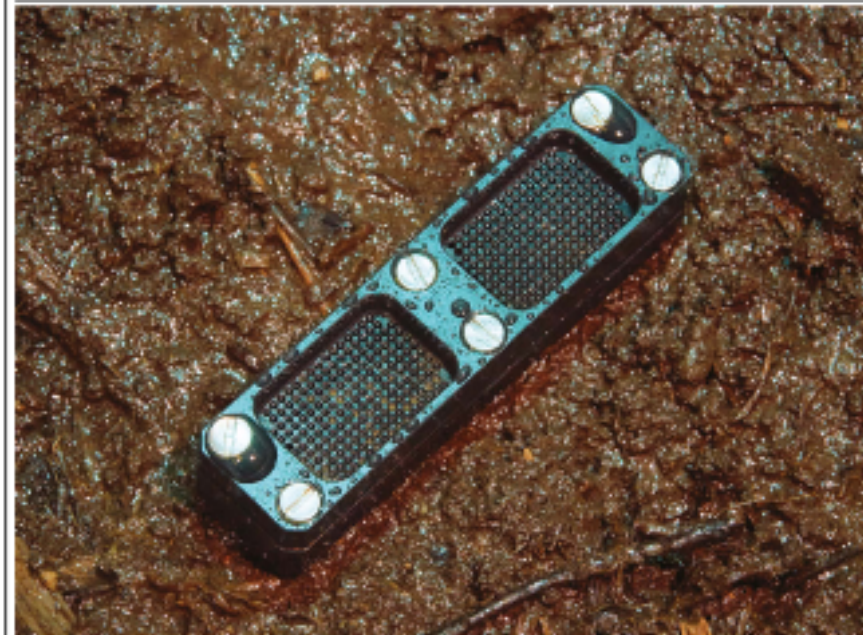
The chip allows researchers to isolate pure cultures of rare organisms in soil.
