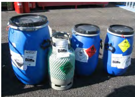
Storage of liquid chemical waste in chemical-resistant plastic containers
